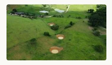
Barraginhas are small, low-cost dams that capture runoff and recharge groundwater. These can be built in sloped, erosion-prone areas.
